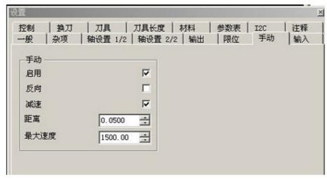
External point switch Enable Hook This feature takes effect after Inverting No hook Acceleration and deceleration After the acceleration and deceleration function hook effect Stepping Minimum step size, how many units to move once more
