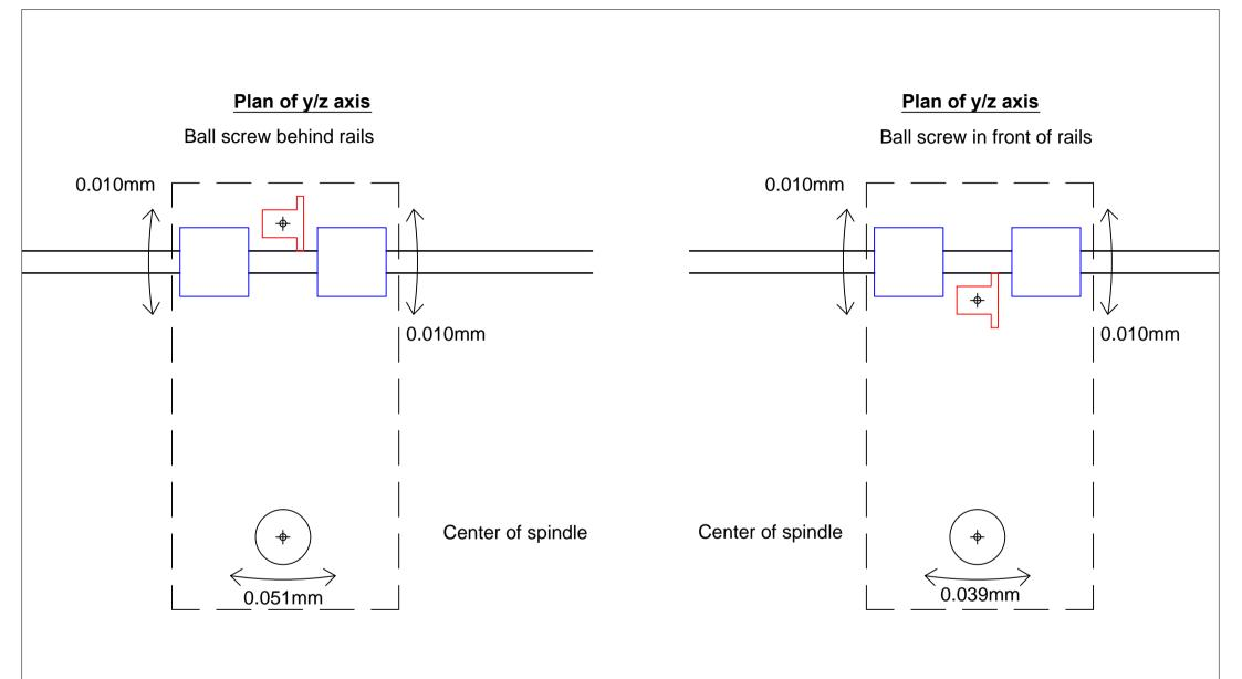
Assuming the ball screw is fixed and provides the pivot point then any radial clearance in the bearings will translate to movement at the spindle nose. placing the ball screw behind the rails increases the lever arm distance and therefore the displacement at the spindle. Note: both arrangements place radial loading on the screw. Optimal ball screw placement is in line with the rails as this minimizes the radial loading.
