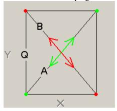
Alternatively, The skew angle (which turns the square into a parallelogram) in degrees can be entered directly. For this, the applicable button has to be selected. If the length radio button is selected, the skew angle which is derived from the A,B, and Q values will be updated upon changing the A, B, and Q values. If these values are invalid, an able of 0 will be displayed.
