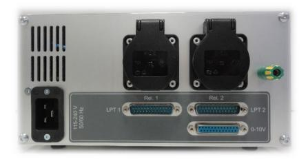
The connection with the controller PC is by means of a 25-pin D-sub connector (LPT = parallel port) on the rear panel. Most signals for basic functions (phase/direction, spindle on/off, etc.) are available on the left connector. The plug-in connector on the controller is male, i.e. to connect it with the PC a 1:1 extension cable with a male/female plug is required. The pins (LPT1) are assigned as follows:
