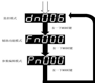
说明：当显示屏显示 Fnxxx,Dnxxx,Pnxxx 时,此时 mode 键为模式切换功能，可直接向其它模式切换，否则 mode 键为返回上层目录功能。Note: when the screen shows Fnxxx, Dnxxx, Pnxxx, mode key at this time as the mode switching function, can be to switched to other mode directly, otherwise the mode key is as the function of returning to the upper directory.
