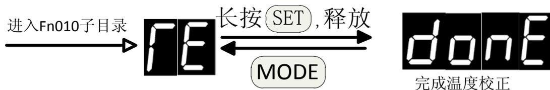
注 1: 进行本操作前, 先用 1.5K 高精度电阻替换温度传感器。Note 1: before the operation, the temperature sensor is replaced with 1.5 K high precision resistor.
