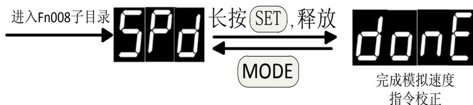
注 1: 在进行校正操作前, 先将 CN2 的模拟电压输入端口 Vref (25 脚) 与 AGND (13 脚) 直接短路。Note 1: before correcting operation, first direct short the CN2 analog voltage input port Vref (25 feet) and AGND circuit (13 feet)
