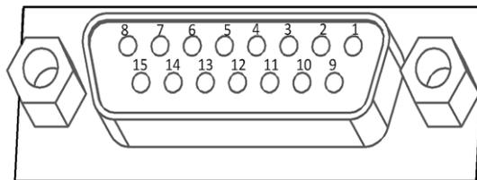
将伺服电机的编码器信号接到伺服驱动器的 CN3 上。Connect the servo motor encoder signal to CN3 of the servo driver.
