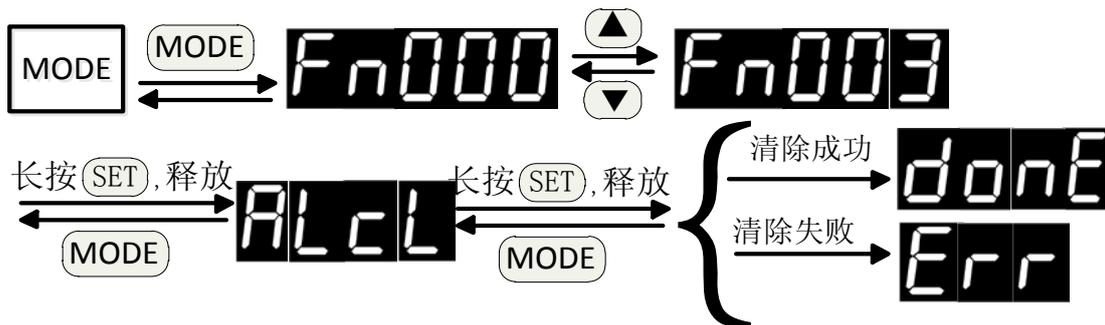
说明：当最后清除失败，显示 **Err**，则检出的报警只有再上电后才可清除。Note:When the clearance is failure at last,display **Err** ,the Checked out alarm can be cleared only after power on again
