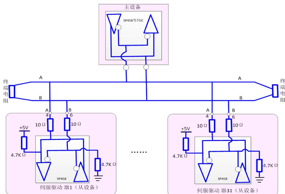
●采用 RS485 通信时，最多可同时连接 31 台伺服驱动器，485 网络末端需分别接一个 120 欧电阻的终端电阻。若欲连接更多的设备，必须用中继器来扩展连接的台数。Adopt RS485 communication, at the same time the most connected and table servo drive, 485 network terminals separately by one euro 120 resistance terminal resistances. If want to connect more equipment, must use Repeaters to expand the connection Numbers
