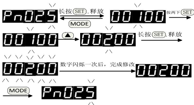
注:Pn025 参数修改后,若没有进行保存操作(Fn001 永久写入),下次上电后,Pn025 参数仍为 100。 Note: Pn025 parameters are modified, if it does not have to save operation (Fn001 immortalised), after the next to electricity, Pn025 parameters still for 100.
