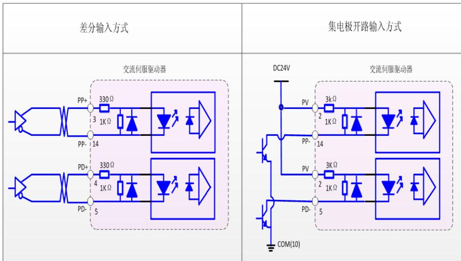
●在差分输入方式下，建议采用 AM26LS31 类似线驱动器；为了使传送的脉冲数据有很好的抗干扰能力，建议采用差分驱动方式；最大输入脉冲频率 500kHz(kpps) 。In the differential input mode, it is recommended AM26LS31 similar line drive; In order to make the transfer of pulse data has good anti-interference ability, it is suggested that the differential drive way; Maximum input pulse frequency 500 KHZ (KPPS).
