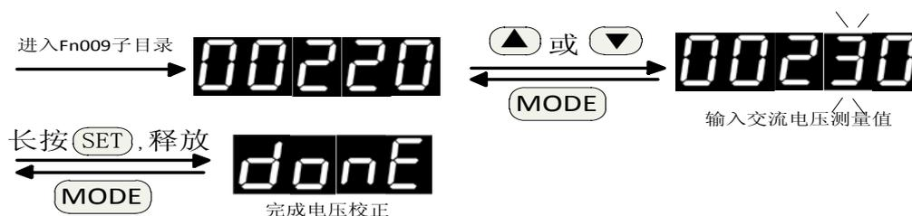
注 1: 在进行校正时, 测量驱动器输入的交流电压, 输入至本操作中。Note 1: when making correction, measurement drive input ac voltage, input to this operation.
