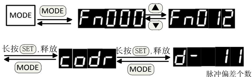
调零操作前，确认电机代码 Pn001 设置值与实际电机型号一致，否则可能导致电机电流过大，损坏电机。调零时，不需要内部使能或外部使能电机，电机将正转几圈，然后锁定零位。当显示的脉冲偏差个数为 0，此时电机已对准零位。Zero before operation, confirm the motor code Pn001 set value and the actual motor model is consistent, otherwise may lead to motor current is too large, damage the motor. Adjust zero, don't need can make internal or external can make the motor, the motor will turn a few laps, and then lock the zero. When the display number of pulse bias of 0, the motor has been aimed at zero.
