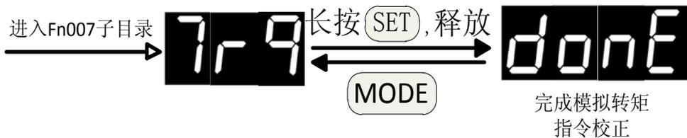
注 1: 在进行校正操作前, 先将 CN2 的模拟电压输入端口 Vref (25 脚) 与 AGND (13 脚) 直接短路。Note 1: before correcting operation, first direct short the CN2 analog voltage input port Vref (25 feet) and AGND circuit (13 feet)
