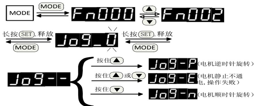
Jog 运行速度与加减速时间可由以下参数设定: JOG The speed and deceleration time is set by the following parameters
