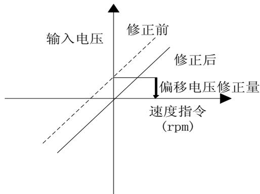
▲ 自动调整偏移，可执行 Fn008 操作。Automatic offset adjusting, perform Fn008 operations.
