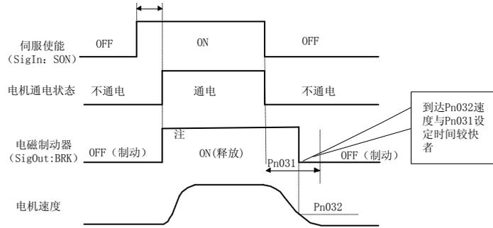
注 1: 使用电磁制动功能时, 伺服断使能方式 Pn004 必须设置为 2 Note 1: when using electromagnetic brake function, servo broken way can make Pn004 must be set to 2
