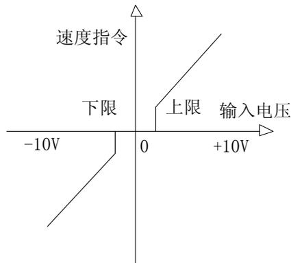
▲ 此时输入电压是经过 PN159 偏移调整后的输入电压。When the input voltage is after adjusting for PN159 offset of the input voltage.
