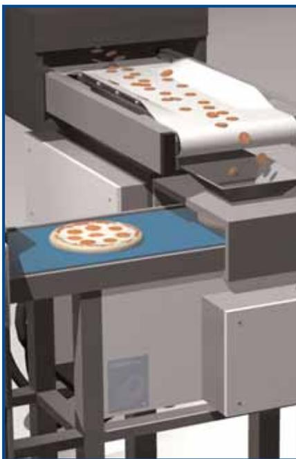
CenterClean belts are constructed with flexible urethane and sealed Kevlar tension members. This construction allows CenterClean belts to be troughed or run on small diameter pulleys with minimal belt stretch.
