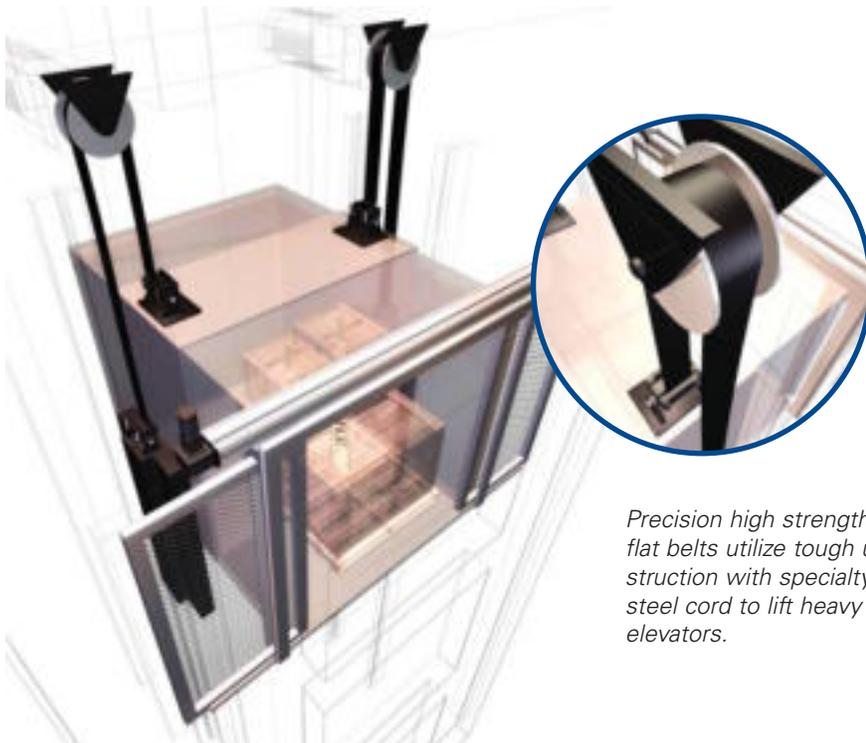
*Precision high strength, low stretch flat belts utilize tough urethane construction with specialty high carbon steel cord to lift heavy loads such as elevators.*
