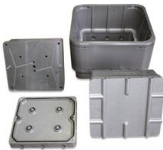
Multi-part thermoform tool system with bucket outer contour and flanges to reinforce the base of the bucket
