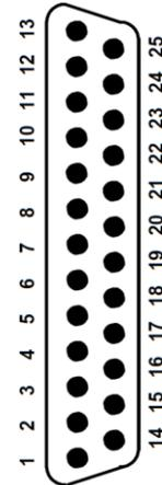
Pin no. 1 is an open-collector signal, i.e. it is switched to ground whenever the spindle motor is switched on and can be used to control (start/stop input) a frequency inverter (max. 30V 50mA). Pin no. 18 is the analog motor speed signal. It is short-circuit-proof so that no damage is caused if a normal LPT cable (Pin 18=ground) is accidentally connected.
