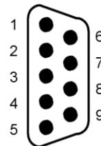
For motors with 3A or higher current a wire gauge of at least 0.5mm<sup>2</sup> (AWG 20) must be used and both pins must always be connected for each wire. For motors with lower current, 0.34mm<sup>2</sup> and one pin are sufficient. Shielding can be connected to either pin 5 or the sheet metal collar of the connector. The motor outputs are short-circuit proof (interturn fault and short circuit).
