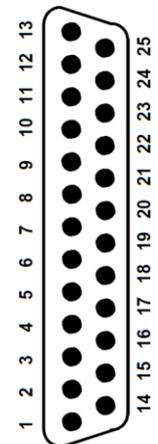
A second LPT port is provided for controlling a tool changer and frequency inverter (see the illustration at the top right). The connector to the PC is male, the one for the tool changer/frequency inverter is female.
