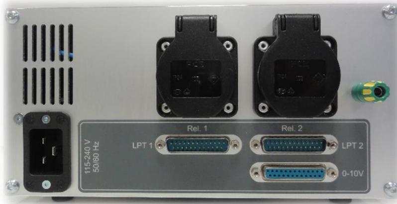
The connection with the controller PC is by means of a 25-pin D-sub connector (LPT = parallel port) on the rear panel. Most signals for basic functions (phase/direction, spindle on/off, etc.) are available on the left connector. The plug-in connector on the controller is male, i.e. to connect it with the PC a 1:1 extension cable with a male/female plug is required.
