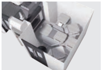
5-station side access turn-type APC OP
