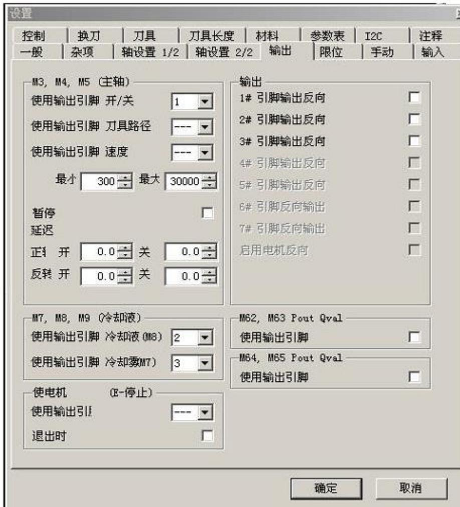
M3,M4,M5 Spindle control command (control spindle function temporarily use)
