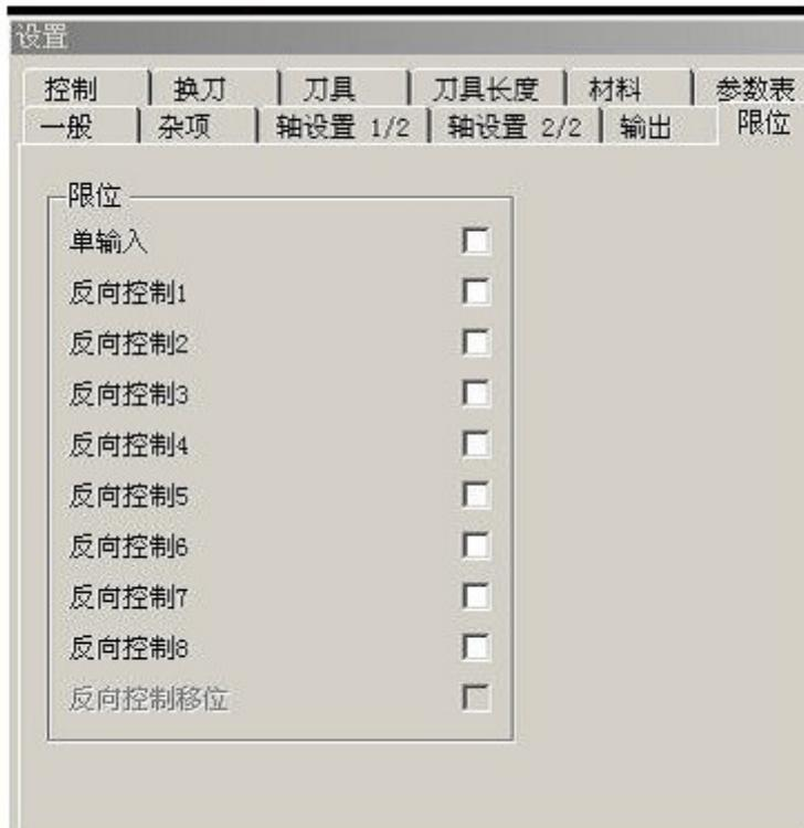
Single Limit: hook after: each axis - + direction limit sharing a port that is restricted to the axis 2 position switch in parallel. Limit one point to the X with, limit 2 to Y, limit 3 to Z, limit 4 to A.
