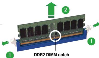
2. Remove the DIMM from the socket.
