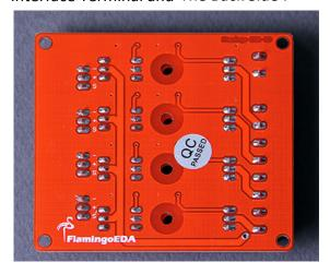
As shown in the picture above, the left side is controlling side. You can input 3~6V signal to trigger the conntrolled switch on the left. Operation is very easy.
