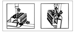
Before removing the protective cover, switch-off the controller and remove the connectors.
