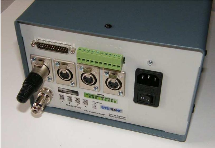
The back panel label shows the positions of the input connections, the axis outputs and pin positions for motor connection.
