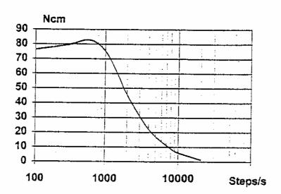
Curve shown with 36V bipolar chopper drive. Windings in parallel. Current 1.4 A/ph.
