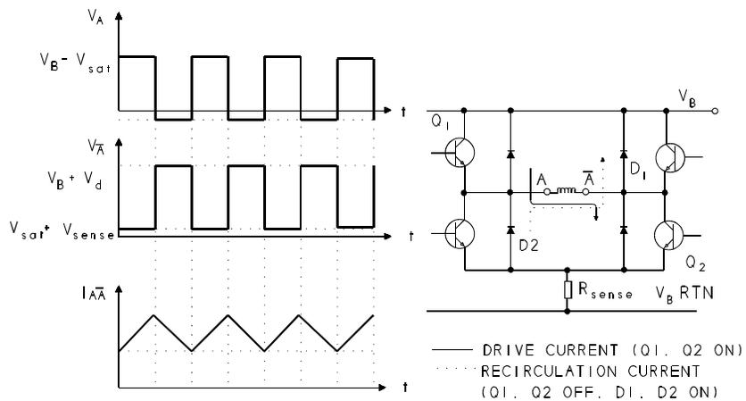
The current decays until the next PWM oscillator pulse turns transistors Q1 and Q2 back on.
