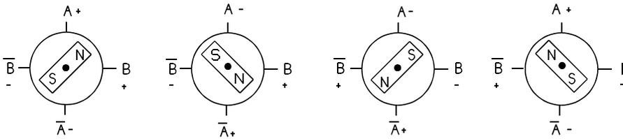
This type of commutation is selected by forcing the  $\overline{\text{HALF/FULL}}$  input low prior to applying power to the module and keeping the input low. The module is now set for Full-step operation. Do NOT change the state of the  $\overline{\text{HALF/FULL}}$  input state during operation since the Full-step or Wave drive mode is selected based upon the state of the module outputs when the  $\overline{\text{HALF/FULL}}$  input is pulled low.
