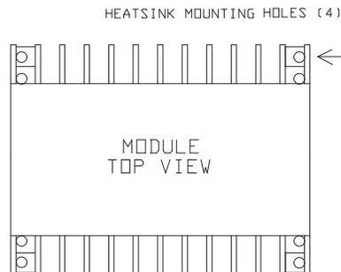
**Note:** Assembly of the self-tapping screws is eased if the diameter of the four mounting holes is increased slightly using a Number 37 drill bit.
