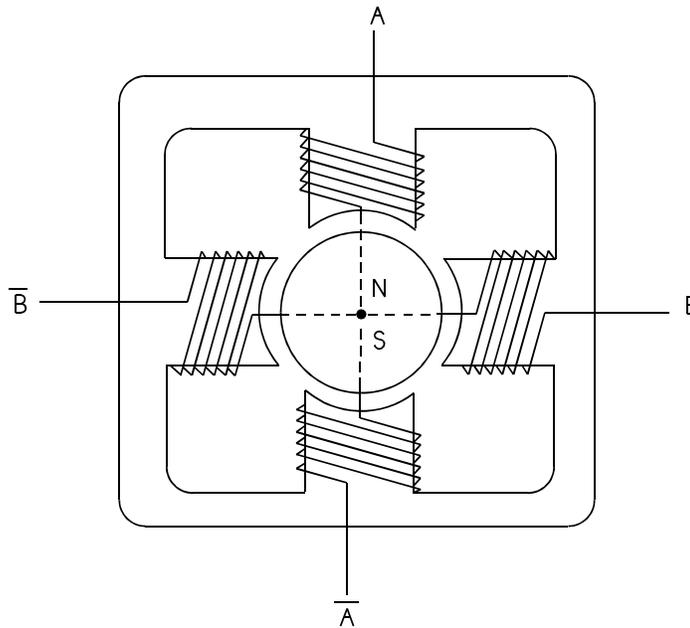
The stator consists of two-phase windings and the rotor is a permanent magnet. The rotor aligns itself with the magnetic field created by the stator windings. By controlling the winding currents in the proper sequence, torque is produced and the rotor will rotate in the desired manner. The phase currents are bidirectional and sequencing of these phase currents is termed commutation. There are three basic types of stepping motor commutation possible with the 5210 module.
