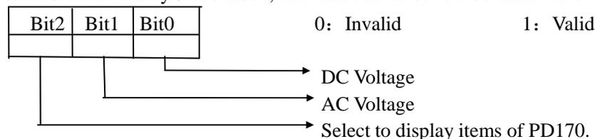
In the contents displayed the factory setting is to show output frequency, set frequency, output current and output revolution through the switch key. If it is necessary to view and monitor other items they can be set through PD170 and PD171.
