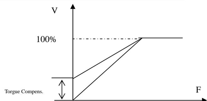
Insufficient compensation will result in the under-torque of the motor at lower frequency. And over compensation will lead to too bigger torque, which will produce a shock to the machine and even result in a trip of the inverter under serious situation.
