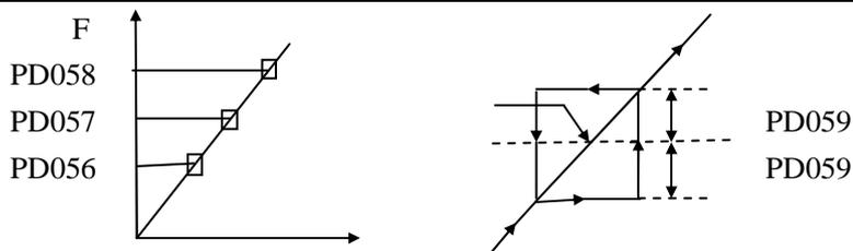
These three frequency skipping points are set for avoiding a mechanical resonance point. In case of PD059=0, all skip frequencies are invalid. The actual skip frequency range is two times that of PD059, as shown in the above diagram.
