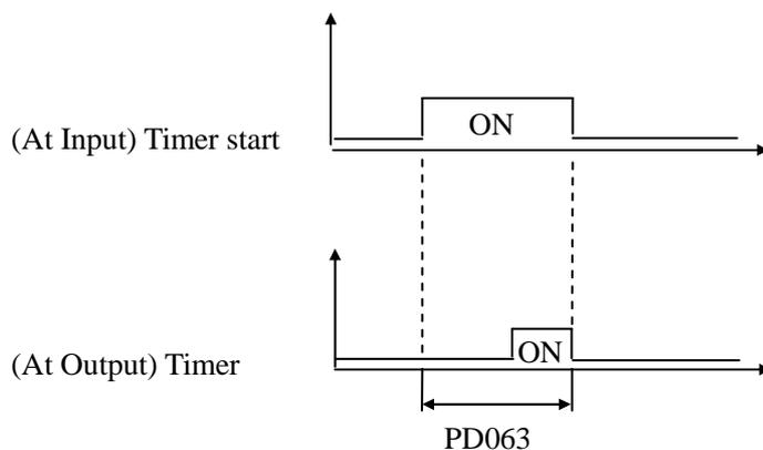
For example, set PD063=5.0s. When the external control terminal (Multi-Input) is valid the output
