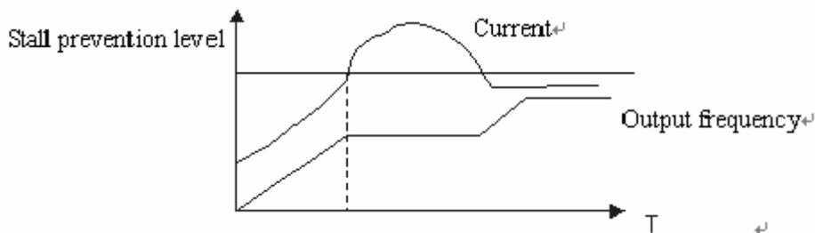
100% current is the rated current of the motor. When this parameter is set to 0, the stall prevention function is invalid.
