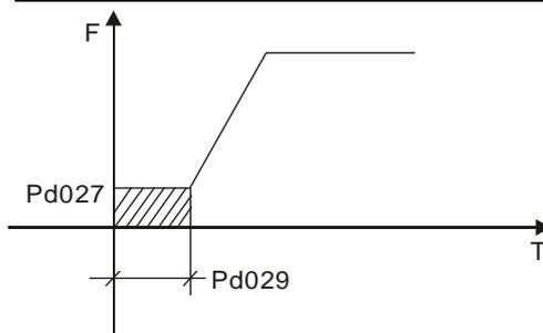
This parameter is set for DC Braking at start and the lasting time of DC Braking current to the motor. If it is set to zero it means DC braking is invalid.
