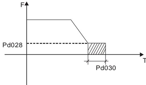
Note: When this parameter is set to any non-zero value it starts DC brake at stop and sends the DC braking time to the motor. DC braking at stop is often used for a high-level stop or positioning control. When this parameter is set to zero it closes DC braking at stop.
