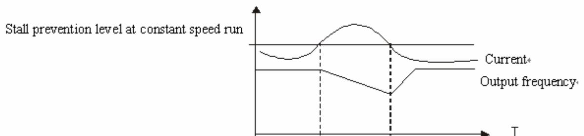
100% current is the Rated Current of the motor. When this parameter is set to 0 the stall prevention function is invalid.
