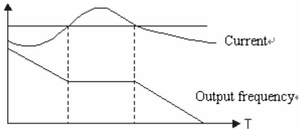
100% current is the rated current of the motor.
