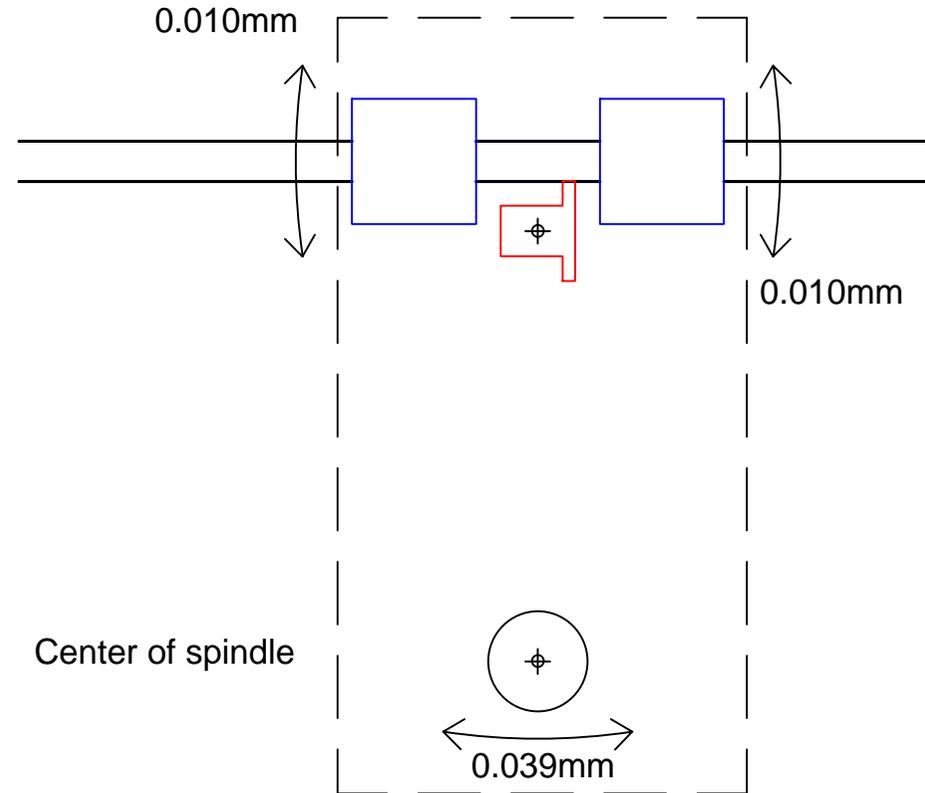
Assuming the ball screw is fixed and provides the pivot point then any radial clearance in the bearings will translate to movement at the spindle nose. placing the ball screw behind the rails increases the lever arm distance and therefore the displacement at the spindle. Note: both arrangements place radial loading on the screw. Optimal ball screw placement is in line with the rails as this minimizes the radial loading. .
