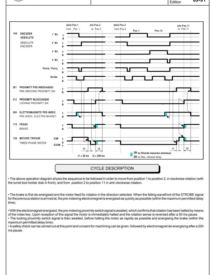
NOTE: The maximum care should be taken regarding the permitted delays, particulary their repeatibility. (delays should be measured directly on the turret component devices).
