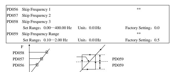
These three frequency skipping points are set for avoiding a mechanical resonance point. In case of PD059=0, all skip frequencies are invalid. The actual skip frequency range is two times that of PD059, as shown in the above diagram.
