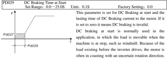
So the DC braking can be executed before starting the motor to prevent the inverter from tripping.
