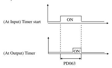
For example, set PD063=5.0s. When the external control terminal (Multi-Input) is valid the output
