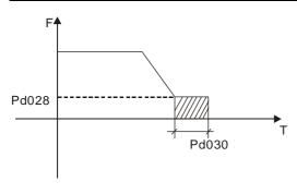
Note: When this parameter is set to any non-zero value it starts DC brake at stop and sends the DC braking time to the motor. DC braking at stop is often used for a high-level stop or positioning control. When this parameter is set to zero it closes DC braking at stop.
