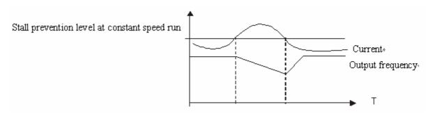
100% current is the Rated Current of the motor. When this parameter is set to 0 the stall prevention function is invalid.
