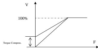
under-torque of the motor at lower frequency. And over compensation will lead to too bigger torque, which will produce a shock to the machine and even result in a trip of the inverter under serious situation.
