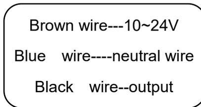
1. As shown on above diagram, connect brown wire of sensor to 10~24V, blue wire to neutral wire, and black wire is output terminal.
